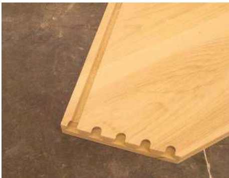
▲ Pic.6 Martin produced the dovetail housings at 45° to the grain but they still retain much of their strength
